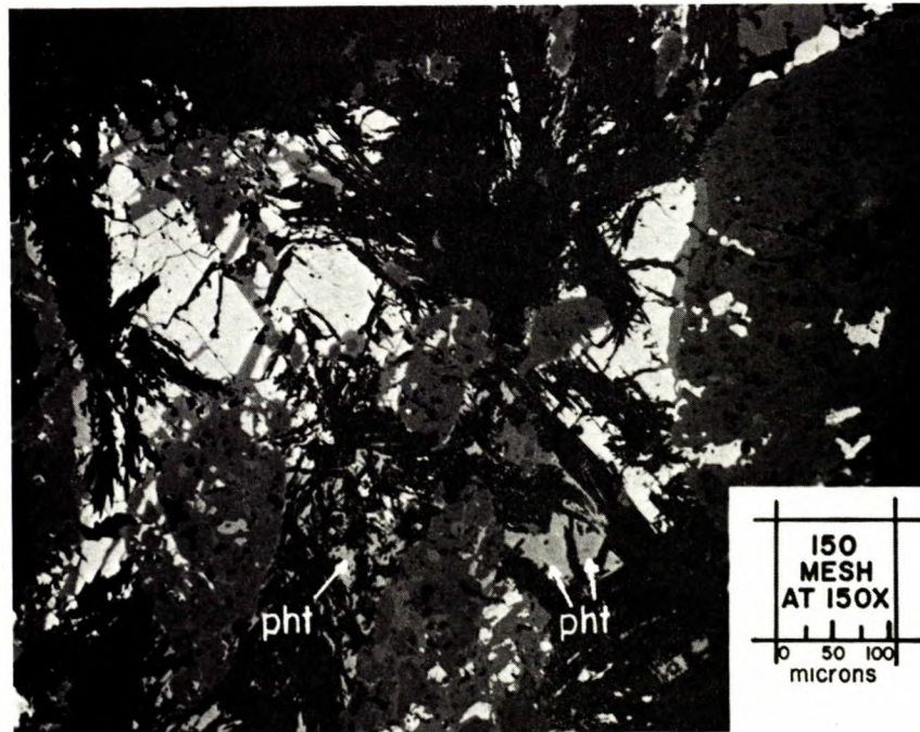
Figure 4. Photomicrograph of a polished section showing grains of chromite (dark grey) with inclusions and rims of magnetite (medium grey), associated with pentlandite (white) and some pyrrhotite (pht) in gangue (black).
