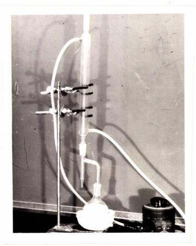
Figure 1. Dean Stark Apparatus for Azeotropic Distillation of Chrysotile Asbestos.
