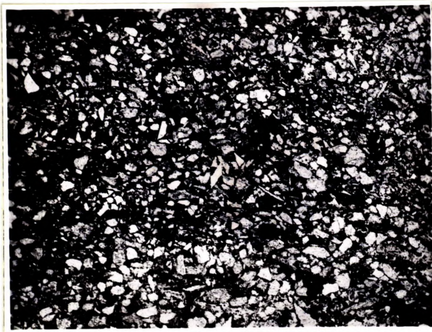
Figure 4. Photomicrograph of brown 'shale', showing abundant fragments of quartz, feldspar (white), altered mafics (pale grey, e.g. A) and calcite (dark grey), imbedded in opaque brownish matrix (black). Polarized light; magnification 50X.
