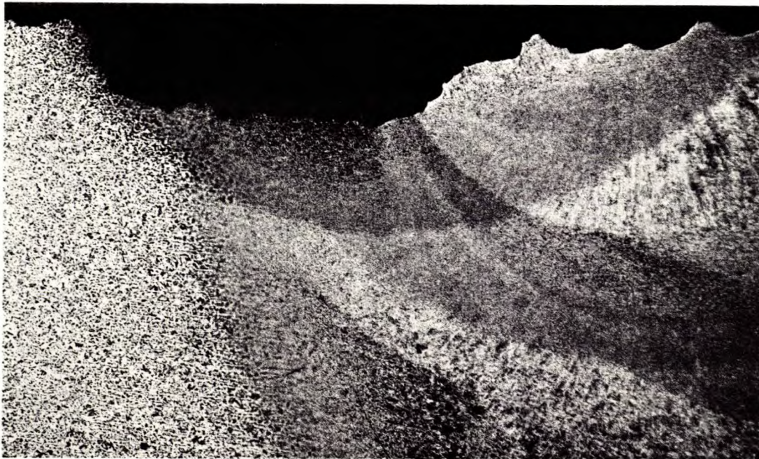
Figure 3. At upper edge of longitudinal weld, on seawater side. Mag. X11.
