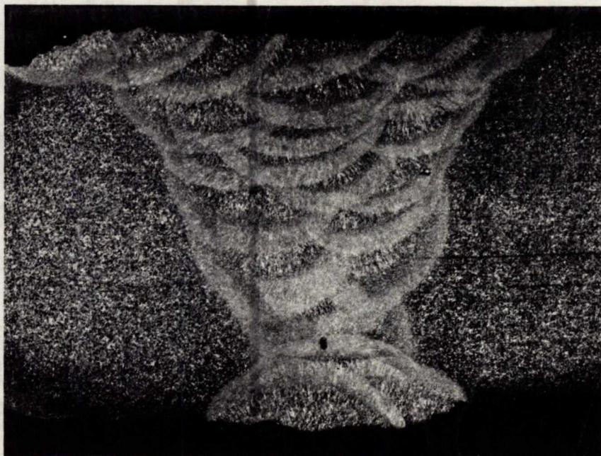
Figure 4. Section from transverse weld with forward edge of the weld when located on the ship at the left and the sea-water side at the top. Mag. X2.
