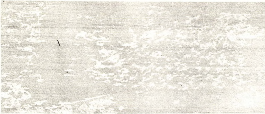
Figure 1. Appearance of surface defects on exterior surface of extrusion, X 1-1/2.
