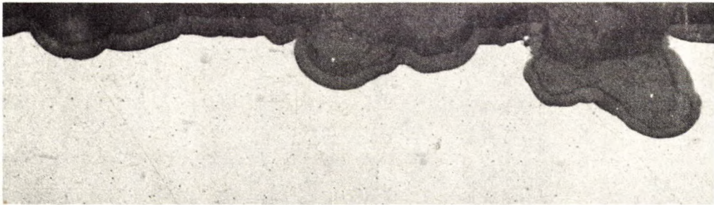
Figure 2. Microstructure of pitted exterior surface. Etched in 0.5% HF, X500.
