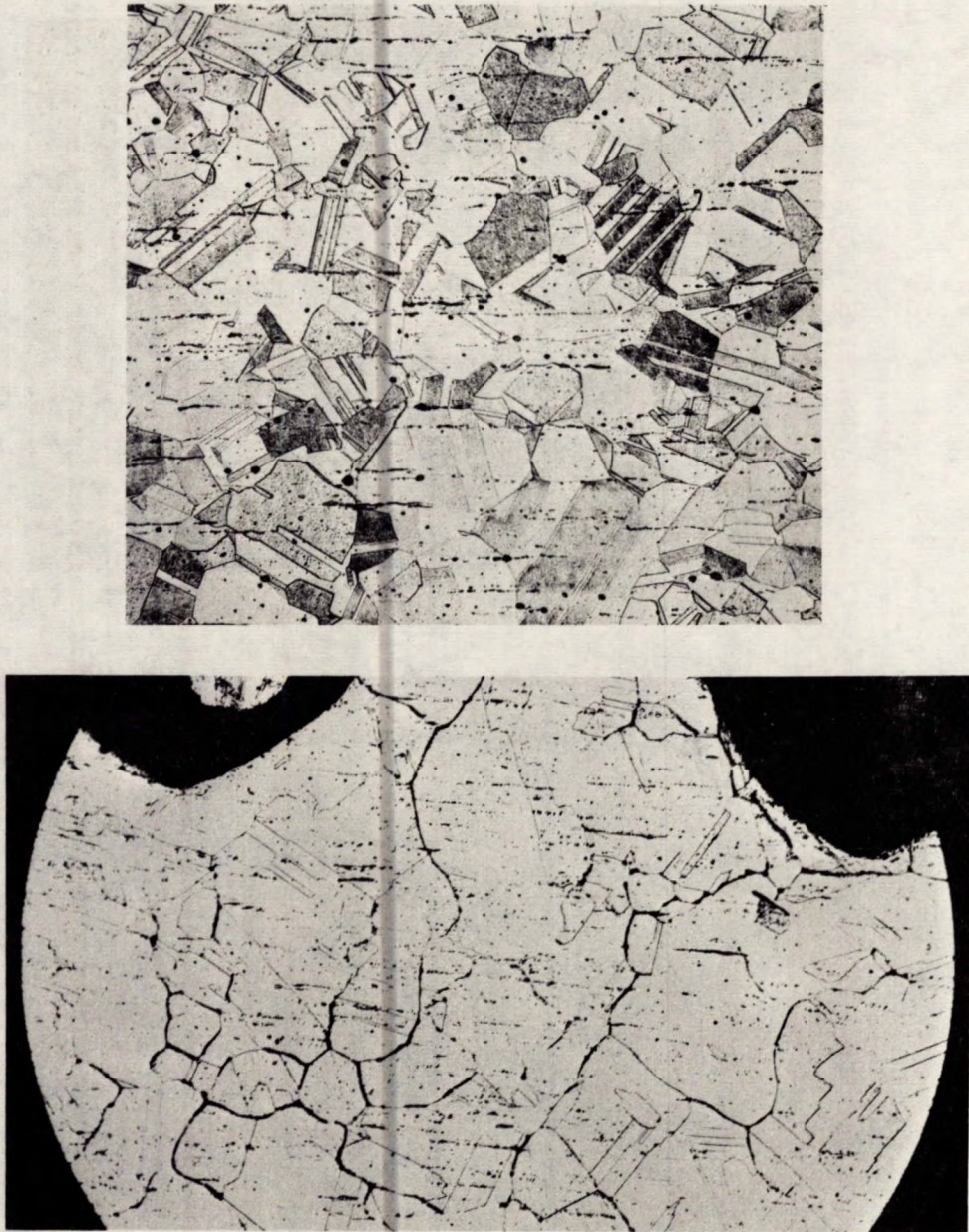
Figure 7. Structures of Inner Capsule No. 5. Electrolytic oxalic etch. (X100)
