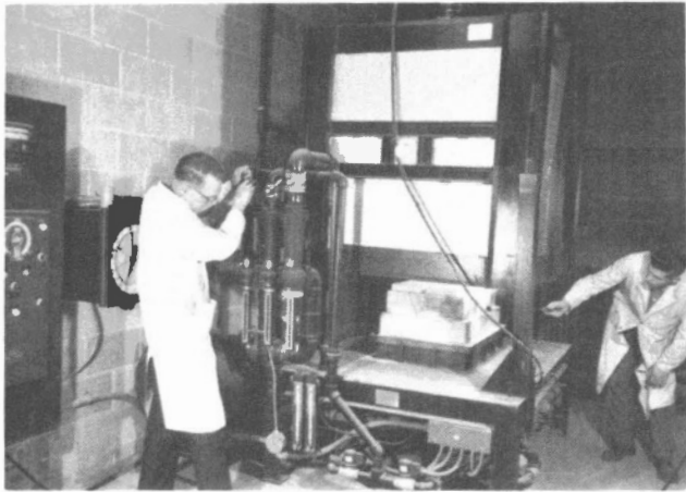
H. Mercier fires brick in Remmey furnace with temperatures to 3500°F
