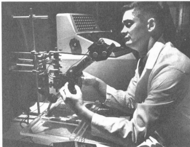
F. Barton measures length distribution of asbestos fibre (Photo - George Hunter)
