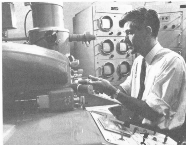
Left - H. Thresh uses the electron probe microanalyzer installed in PMRL in 1964. This instrument makes possible identification of final dispersed compounds in an alloy (Photo - George Hunter); Right - D.R. Bell uses quantitative TV metallographic microscope (Photo - George Hunter)
