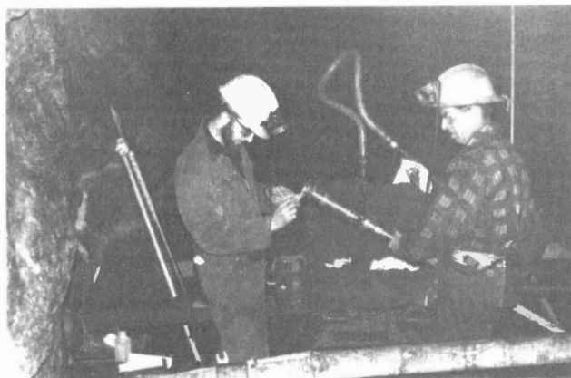
R. Miller (left) prepares "doorstopper" strain cell for installation in a borehole, Nordic mine, Elliot Lake, Ontario
