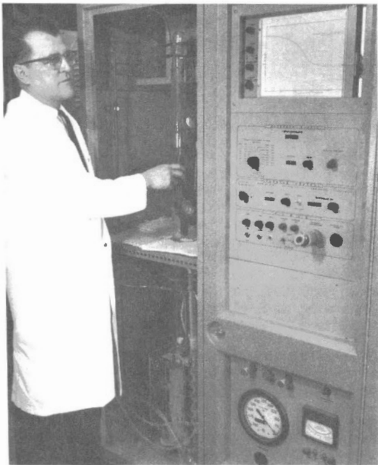
P. Marier carries out kinetic decomposition studies using automated analytical equipment.
