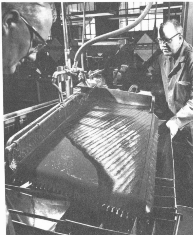
H. Renaud and R. Bruce conducting gravity concentration test
