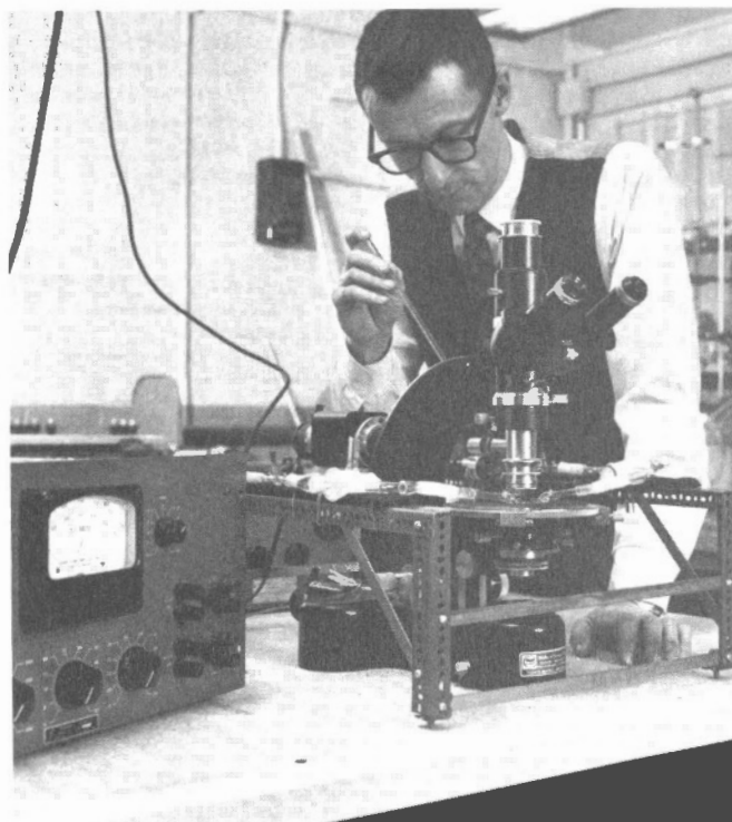
L. Sirois determines electrical characteristics of minerals in flotation research (Study of electrophoresis) (Photo - George Hunter)
