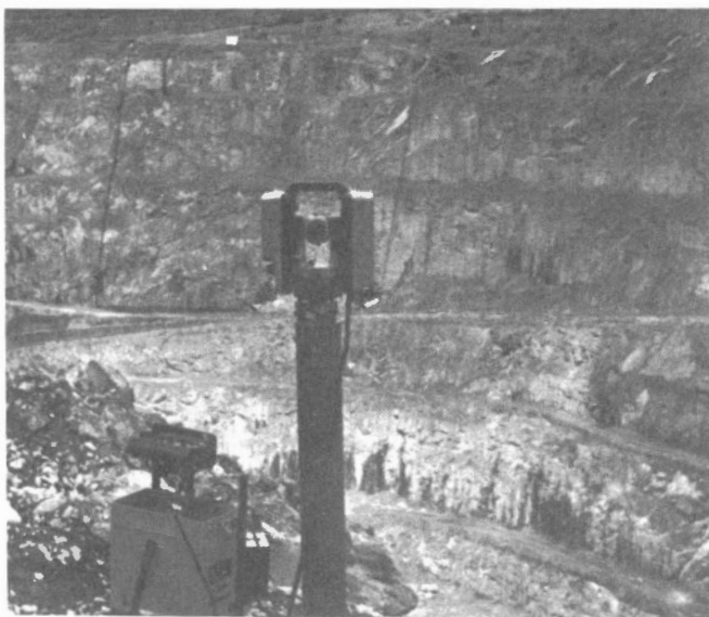
Laser-theodolite mounted on GSC-type monument at Kidd Creek open pit mine. Used to measure distance and angles in connection with ground movement monitoring
