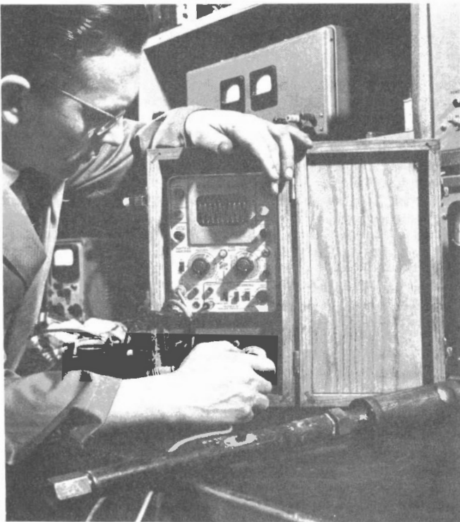
F. Kapeller adjusts instrument to measure sonic velocity in rock
