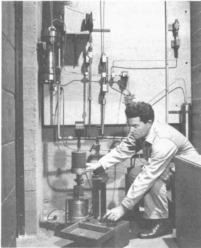
R.E. Carson checks high pressure porosimetry plant related to catalysis research (Photo - George Hunter)
