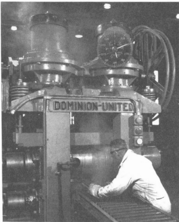
A. Baker adjusts magnesium slab during rolling operations
