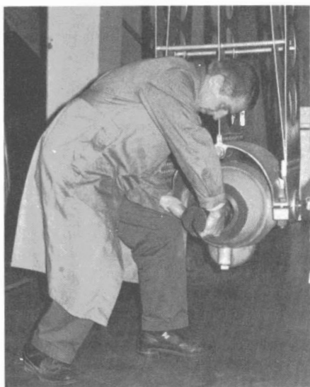
P. Larsen determines the power rating of an explosive sample, 1968
