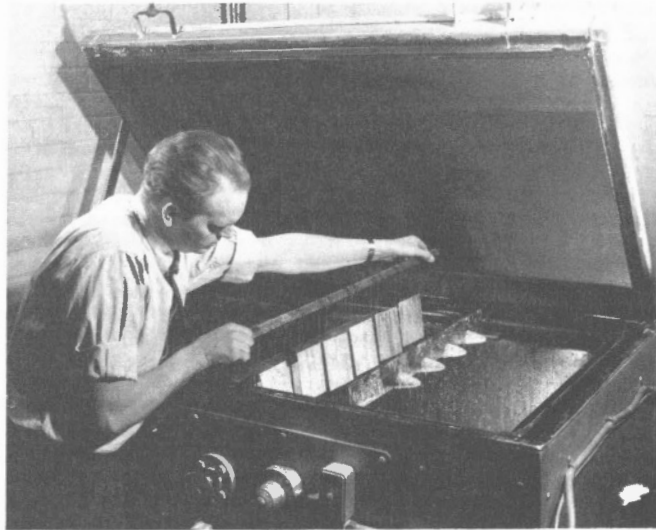
W. Dingley inspects samples in earlier accelerated marine corrosion test (Photo - NFB)
