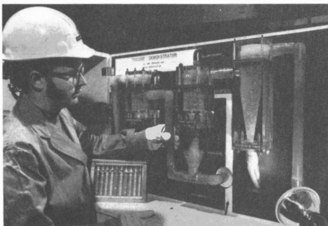
N.E. Anderson operates a demonstration model of a two-stage water coal-washing cyclone using synthetic coal, Western Regional Laboratory (Photo - George Hunter)
