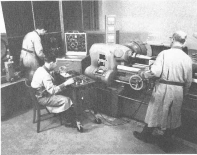
R. Beer, M. Séguin and S. Samson operating machinability research lathe with recording (x,y) instruments and tool post dynamometer
