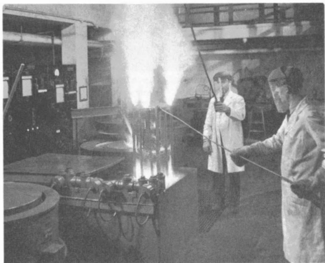
H. Fairfield and J. Kosowan quench drill steel rods at 1550°F in oil bath (Photo - NFB)
