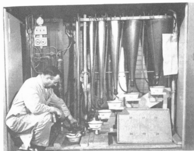
H.R. Renaud performing size analysis on ore sample using the Haultain Infracizer, circa 1960
