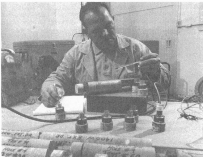
J. St. Onge carries out laboratory measurements following field stress investigations; Leeman doorstopper stress gauges shown
