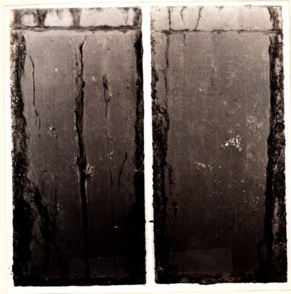
SAMPLES 674 WITH ONE PRIMER AND TWO TOP COATS OF PAINT, AFTER 90 DAYS IN SALT SPRAY CABINET.
