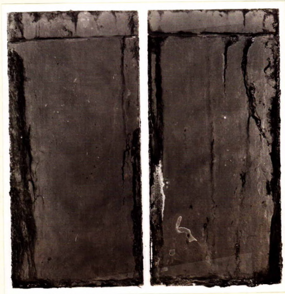
SAMPLE 674 WITH ONE PRIMER AND THREE TOP COATS OF PAINT, AFTER 90 DAYS IN SALT SPRAY CABINET.
