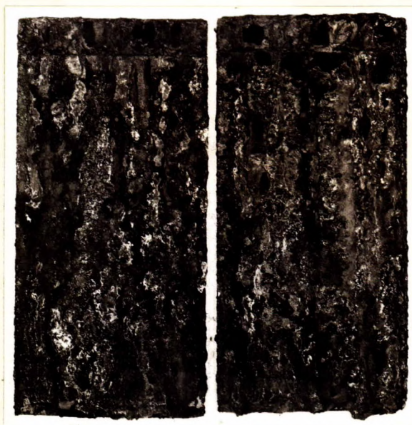
SAMPLE 740 WITH TWO COATS OF PAINT, AFTER 90 DAYS IN THE SALT SPRAY CABINET.
