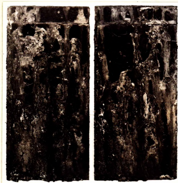
SAMPLE 740 WITH THREE COATS OF PAINT, AFTER 90 DAYS IN THE SALT SPRAY CABINET.
