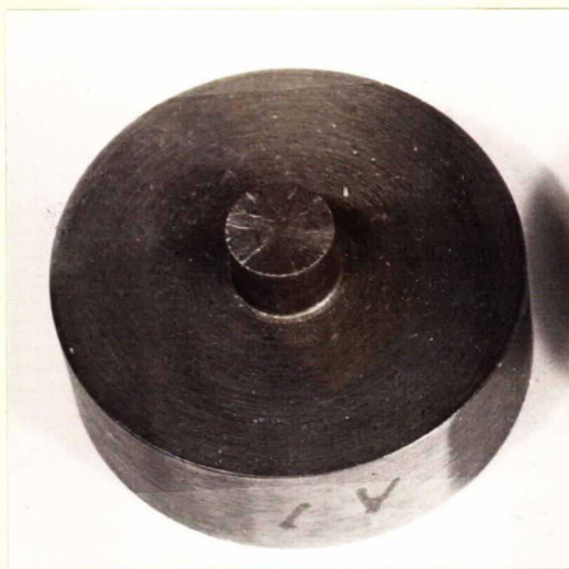
ROTTER MACHINE IMPACT ANVIL.
