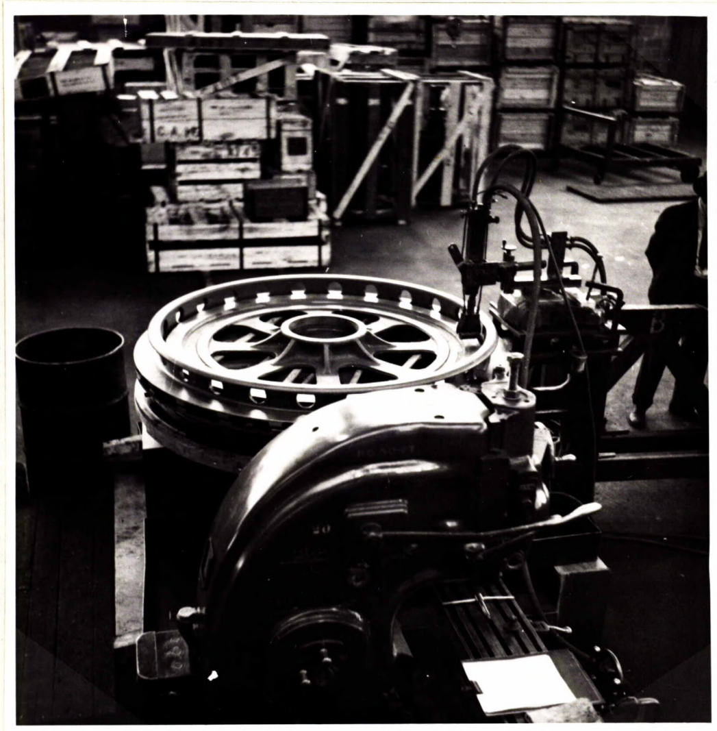
ARRANGEMENT OF RACER PLATE AND FLAME-HARDENING EQUIPMENT FOR FLAME HARDENING.
