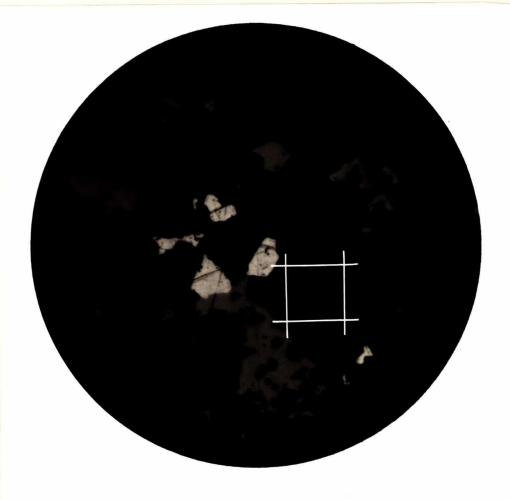
PHOTOMICROGRAPH OF POLISHED SECTION SHOWING NATIVE GOLD (WHITE) ALONE IN GANGUE (BLACK) AND AGAINST CHALCOPYRITE (GREY).
