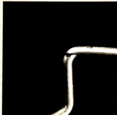
THE FRACTURE AT POINT A, (Note deformation on inside of the bend)
