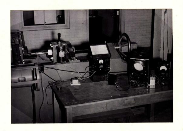
APPARATUS USED FOR THE DYNAMIC CALIBRATION WITH STRAIN GAUGES.
