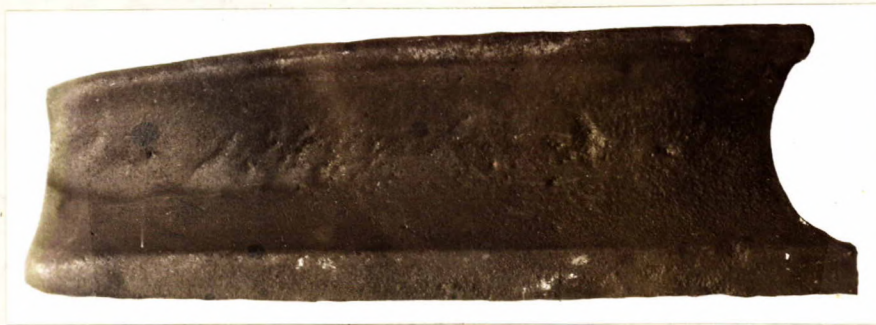
MANGANESE STEEL CASTING, SHOWING WORN INSIDE SURFACE.
