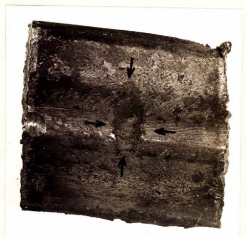
ROLLED SECTION. Showing cavity defect encountered in rolling.
