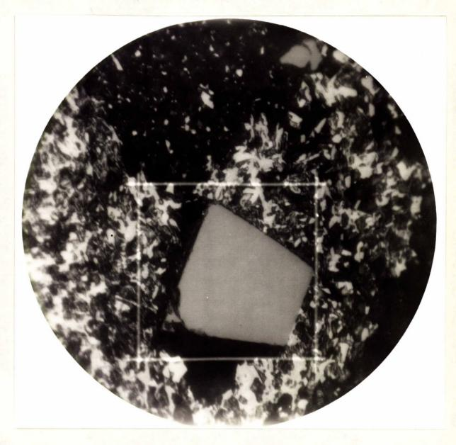
Central part of field shown in Figure 2, at higher magnification to show better the relationship of the ore minerals. A 200-mesh Tyler screen opening is superimposed. The magnification is 900X.
