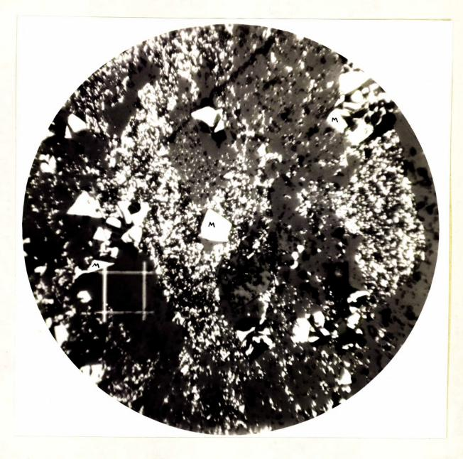
Shows an average field in polished section prepared from sample of Attikamagen iron ore, with a 200mesh Tyler screen opening superimposed at 200X.
