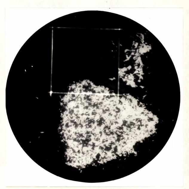
Photomicrograph of a polished section of flotation concentrate from Lake Attikamagen iron ore, showing grains of hematite (white) highly impregnated with finely divided gangue (grey). Pits and bakelite are dark grey to black. The magnification is 800X. A 200-mesh Tyler screen opening is superimposed.
