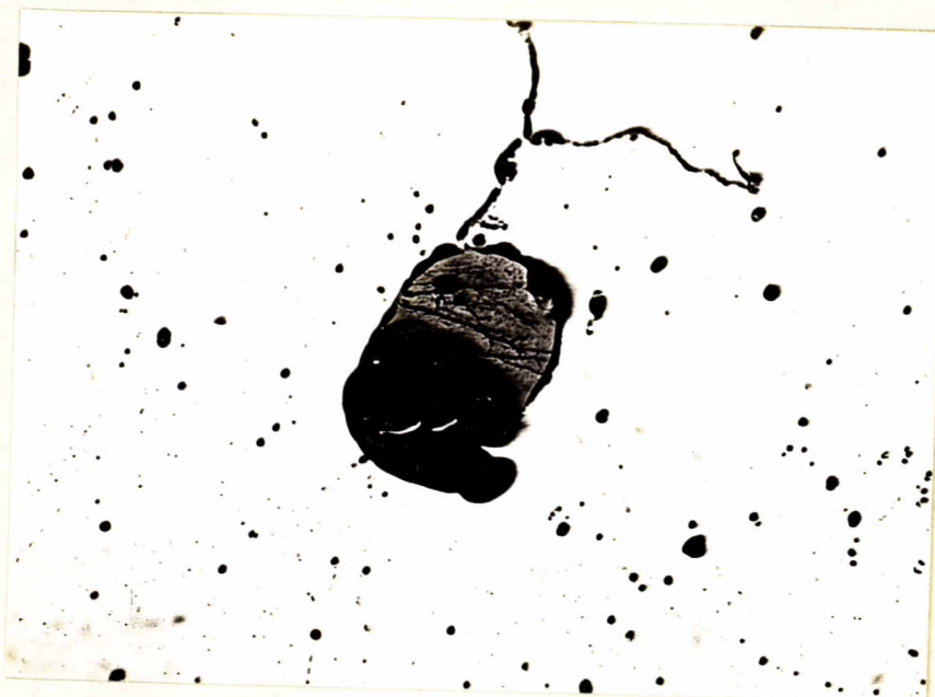
X100, nital etch. Showing large inclusions.
