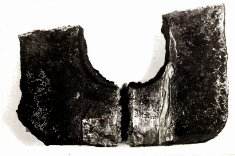
MANGANESE STEEL SWING HAMMER CRACKED IN THE MOULD.
