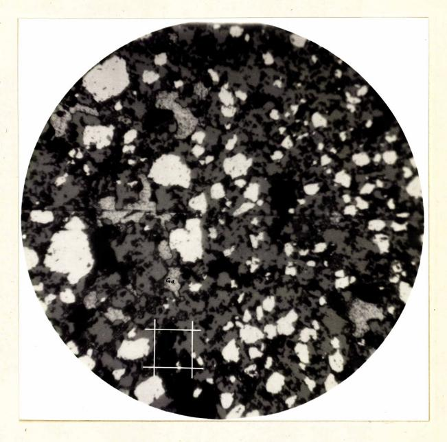
PHOTOMICROGRAPH OF AN AVERAGE FIELD IN THE POLISHED SECTIONS MADE FROM SAMPLE NO. 2 ("STEEL-GALENA" ORE), SHOWING GRAIN SIZES AND GENERAL CHARACTER OF THE MINERA-LIZATION. A 200-MESH TYLER SCREEN OPENING IS SUPER-IMPOSED.
