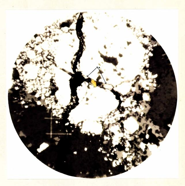
PHOTOMICROGRAPH OF POLISHED SURFACE, SHOWING A SMALL GRAIN OF GOLD (YELLOW) ALONG A FRACTURE IN PYRITE (WHITE) AND GENERAL CHARACTER OF THE MINERALIZATION IN SAMPLE NO. 1.
