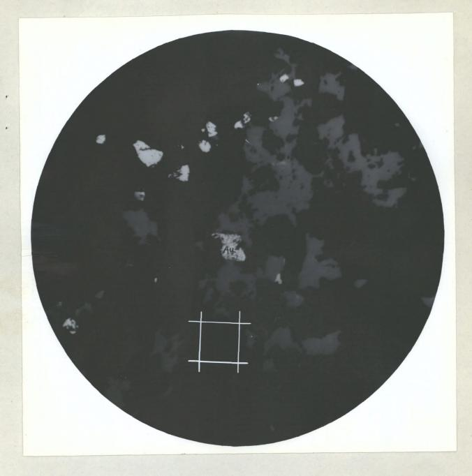
PHOTOMICROGRAPH OF POLISHED SURFACE, SHOWING A GRAIN OF GOLD ASSOCIATED WITH SPHALERITE IN SAMPLE NO. 3. A 200-MESH TYLER SCREEN OPENING IS OUTLINED IN WHITE.
