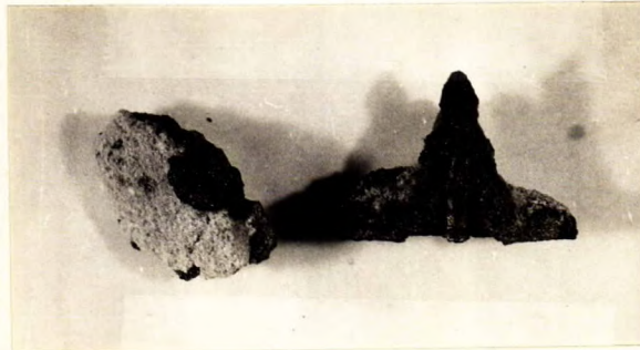
FORMATION OF IRON SILICATE AROUND CHAPLETS.
