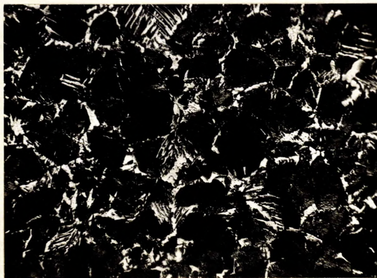
X500, nital etch. FLAME-HARDENED AREA, SHOWING PROEUTEC- TOID FERRITE (WHITE) CAUSED BY IMPROPER COOLING RATE.
