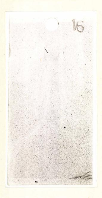
CONDITION OF TYPICAL PANEL COATED WITH A MIXTURE CONTAINING SHELL OIL CO. PREVENTIVE COMPOUND, AFTER HYDROBROMIC ACID NEUTRALIZATION TEST.
