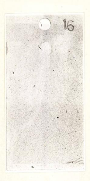
STEEL PANEL AFTER HYDROBROMIC ACID NEUTRALIZATION TEST IN WHICH THE EMULSION CONTAINED McCOLL-FRONTENAC LUB. OIL AND THE NEUTRALIZING MIXTURE CONTAINED SHELL PREVENTIVE COMPOUND WITH OIL FROM THE R.C.A.F. AS DILUENT.
