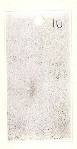
STEEL PANEL AFTER HYDROBROMIC ACID NEUTRALIZATION TEST IN WHICH THE EMULSION CONTAINED THE LUB. OIL FROM THE R.C.A.F. AND THE NEUTRALIZING MIXTURE CONTAINED IMPERIAL OIL PREVENTIVE COMPOUND WITH STANOLAX AS DILUENT.
