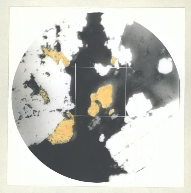
PHOTOMICROGRAPH OF POLISHED SECTION SHOWING GRAIN SIZE AND MODES OF OCCURRENCE OF NATIVE GOLD IN SAMPLE.
