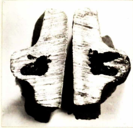
SHRINKAGE CAVITY AT A, FIGURE 2. (Approximately twice actual size).
