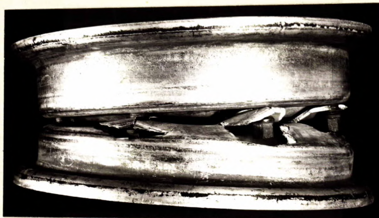
SIDE VIEW OF DAMAGED ALUMINIUM ALLOY TRUCK WHEEL.
