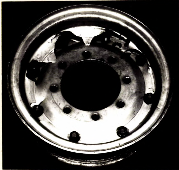
TOP VIEW OF DAMAGED ALUMINIUM ALLOY TRUCK WHEEL. (Approximately 1/6 actual size).
