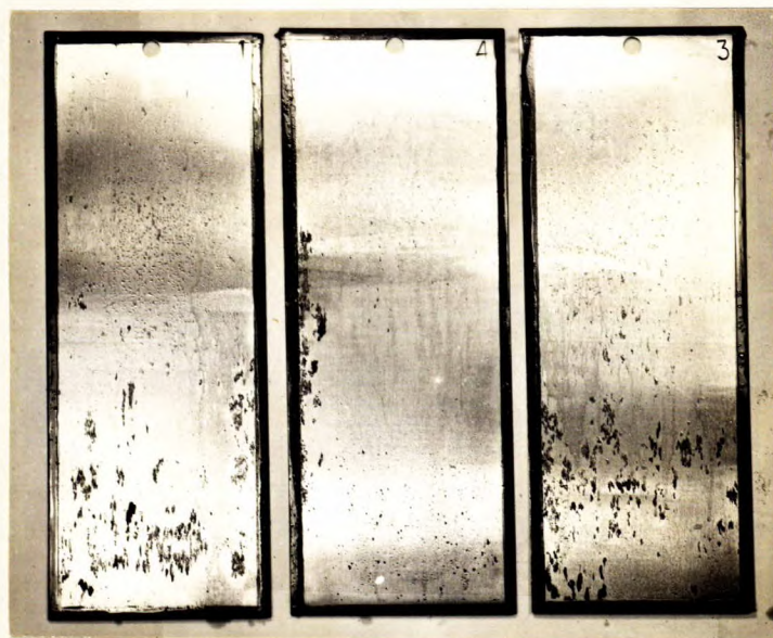
EMIERED SIDES OF TYPICAL STEEL PANELS COATED WITH SHELL ENSIS FLUID 211, AFTER TESTING FOR 150 HOURS IN THE DYNAMIC HUMIDITY CABINET.
