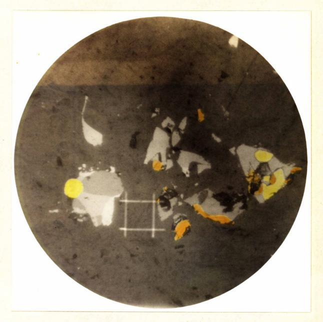
PHOTOMICROGRAPH OF POLISHED SECTION OF TWICE CLEANED COPPER-LEAD CONCENTRATE.
