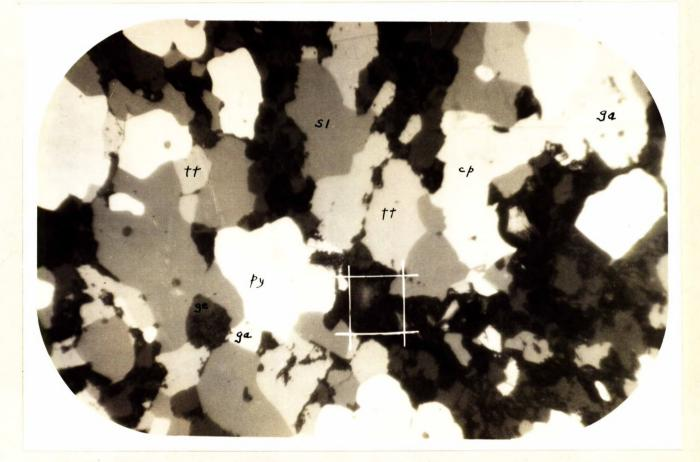
PHOTOMICROGRAPH OF POLISHED SECTION, SHOWING THE GENERAL RELATIONSHIPS OF THE ORE MINERALS IN HAND SAMPLES FROM BIG BULL PROPERTY, TAKU RIVER, B.C.
