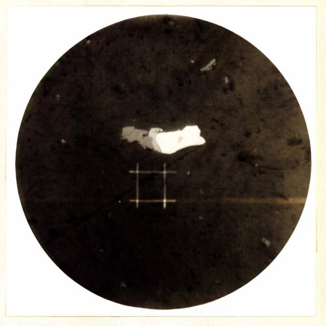
PHOTOMICROGRAPH OF POLISHED SURFACE, SHOWING A COMBINED GRAIN OF PYRITE, GREY COPPER AND SPHALERITE IN A CLEANED ZINC CONCENTRATE.
