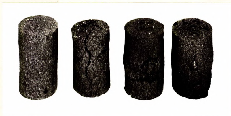
A B C D SAND SPECIMENS SUBJECTED TO THE SHOCK TEST.
