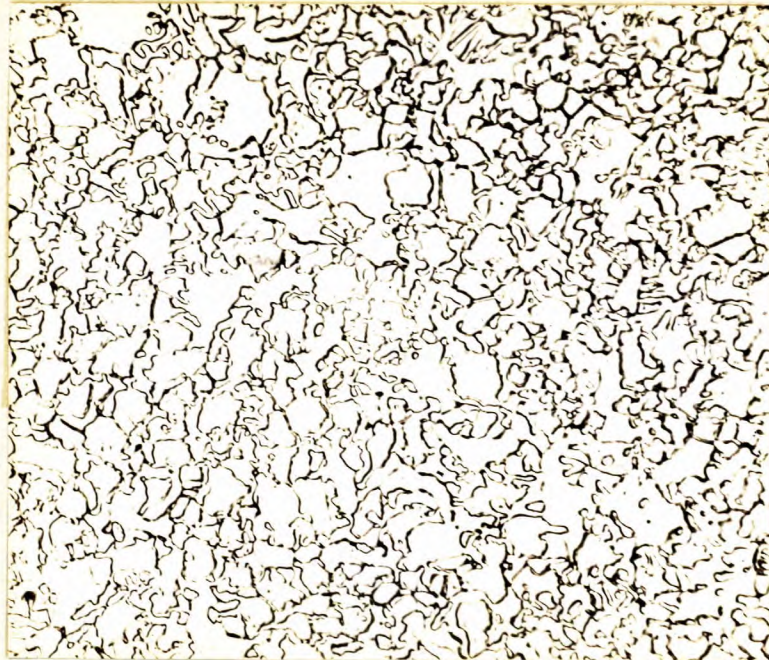
X1000, Vilella's etch.* SILCHROME X.C.R. VALVE. Ferrite and austenite.
