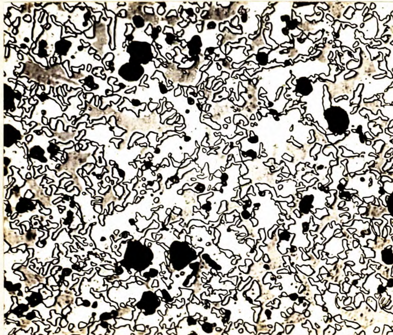
X1000, ferricyanide etch.** SILCHROME X.C.R. VALVE. Ferrite and austenite. The black areas are probably etching pits.
