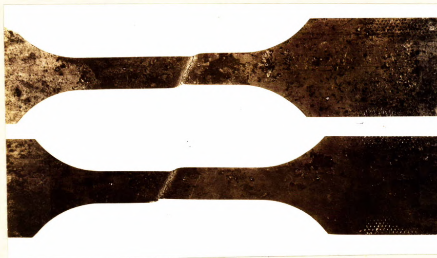
FRACTURES IN 1/8-INCH BULLETPROOF PLATE TEST SPECIMENS.
