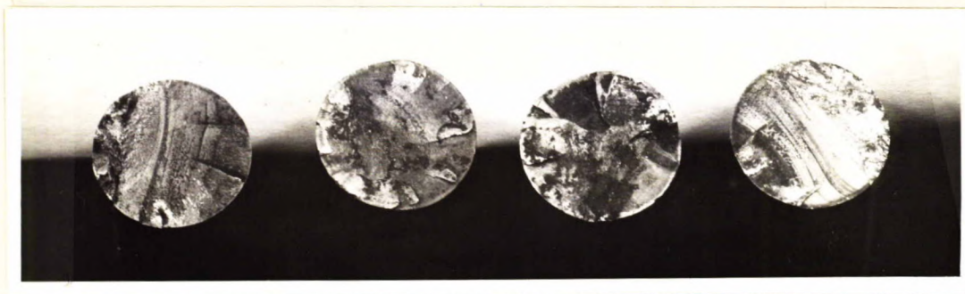
FRACTURE SURFACES TYPICAL OF FATIGUE FAILURES.
