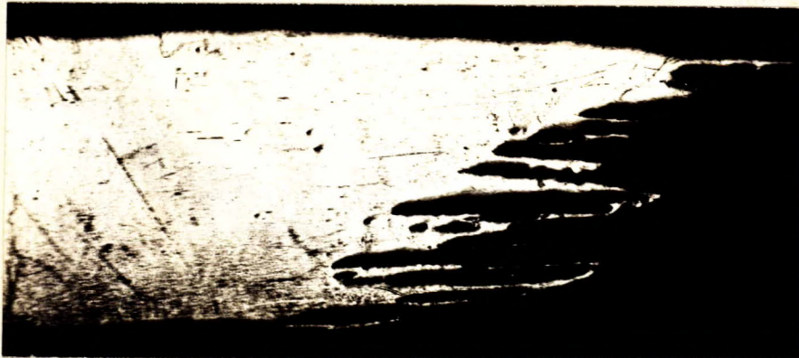
X32. Section "A". SHOWING DUCTILE NATURE OF FRACTURE IN TUBING.
