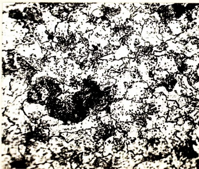
X1000, nital etch. SECTION "A" AT BREAK. Ferrite, pearlite, and carbides.
