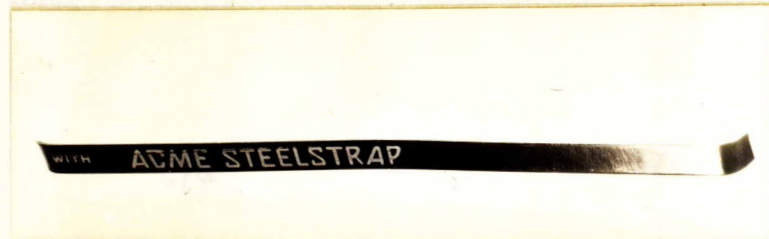
ENAMELLED STEEL STRAP BEFORE CORROSION TEST.
