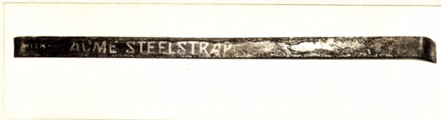
ENAMELLED STEEL STRAP AFTER 42 HOURS IN THE 20 PER CENT SALT SPRAY AT 95° F. (35° C.).
