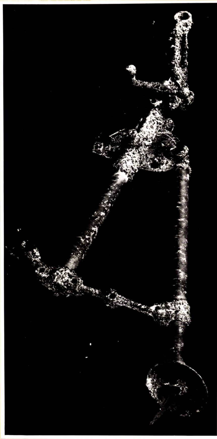
UNTREATED SECTION OF LIGHTENED BIPOD, CONSISTING OF MAGNESIUM, ALUMINIUM AND IRON PARTS. AFTER 200 HOURS IN THE 5 PER CENT SALT (SODIUM CHLORIDE) SPRAY AT 95° F. (35° C.). UNCLEANNED.
