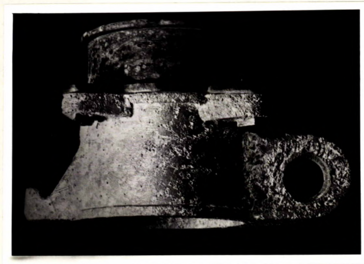
MAGNESIUM SLEEVE (BOTTOM) BOLTED TO BRASS SLEEVE (TOP) FROM WHICH IT IS SEPARATED BY A NON-METALLIC GASKET. AFTER SALT SPRAY TREATMENT AND CLEANING.
