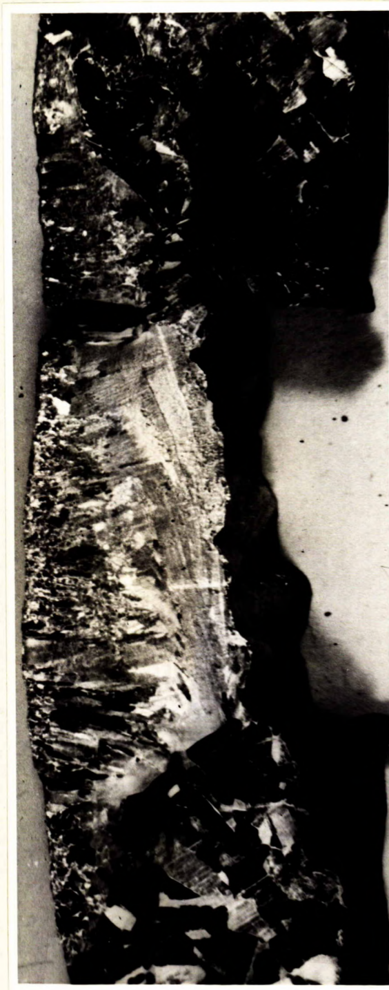
TRANSVERSE SECTION OF WELD REPAIR AREA, ETCHED IN AQUA REGIA.
