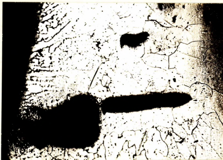
X50, aqua regia and glycerine etch. LACK OF FUSION BETWEEN ENDS OF SHEET. (Area B).
