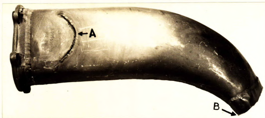
GENERAL VIEW OF INCONEL EXHAUST STUB, SHOWING CRACKS ALONG WELDS AT A AND B.
