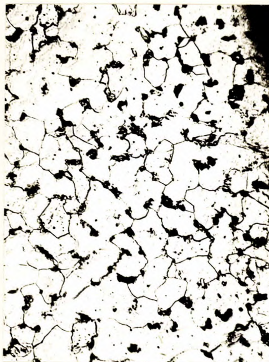
X250, nital etch. TYPICAL OF METAL NEAR OUTSIDE SURFACE.
