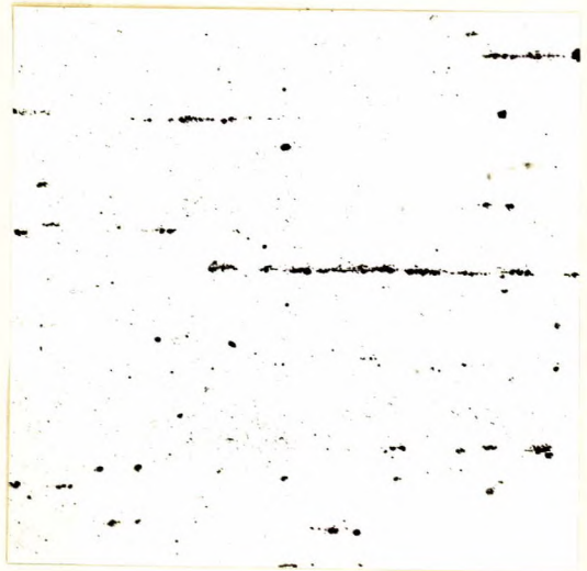
X100, unetched. SHOWING INCLUSIONS.
