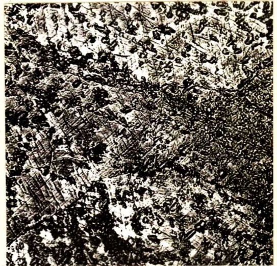
X200, nital etch. MICROSTRUCTURE \frac{1}{4} INCH FROM SURFACE.
