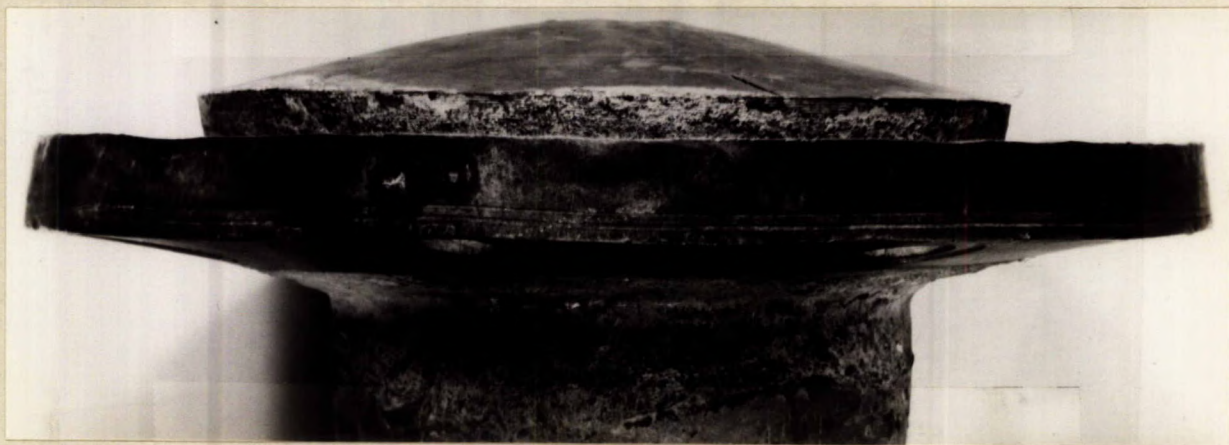
PIPE PRESSURE TEST ASSEMBLY AFTER TESTING. Note pronounced outward expansion of end cover plate.
