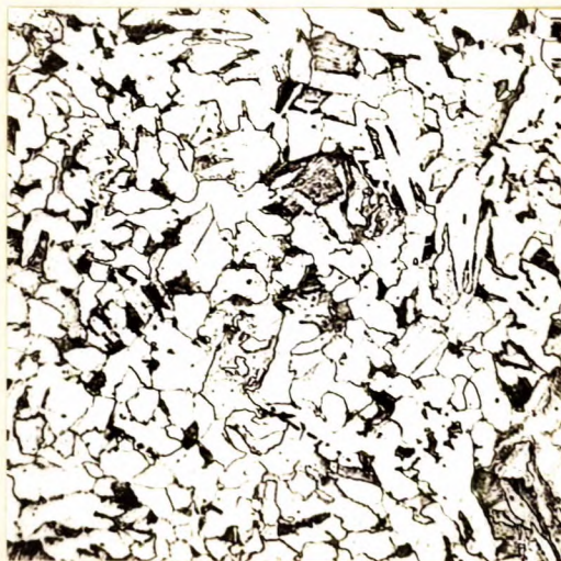
X250, nital etch. TUBING IN "NORMALIZED" CONDITION.
