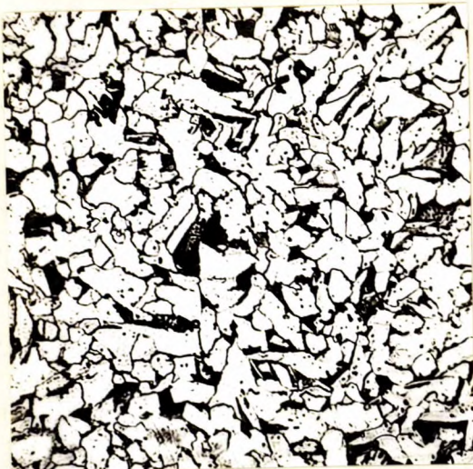
X250, nital etch. Portion unaffected by necking.
