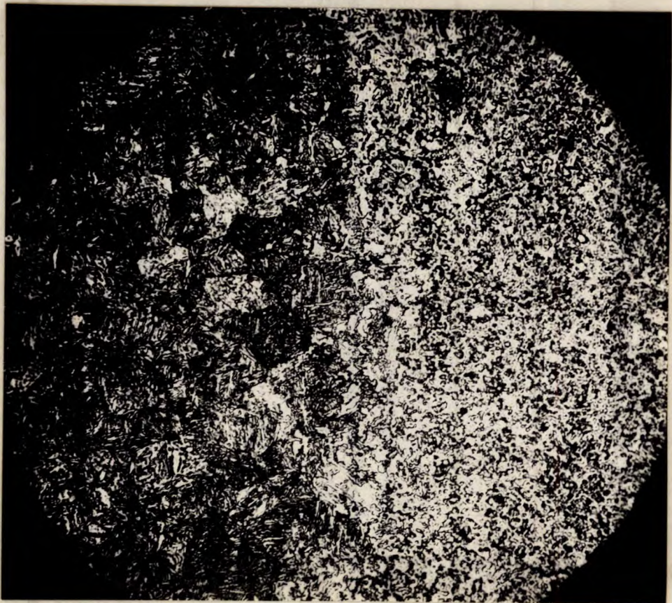
X500, etched in 1 per cent HCl and 4 per cent picric acid in alcohol. TRANSITION ZONE OF BULLETPROOF PLATE. Note spheroidizing effect on carbides.
