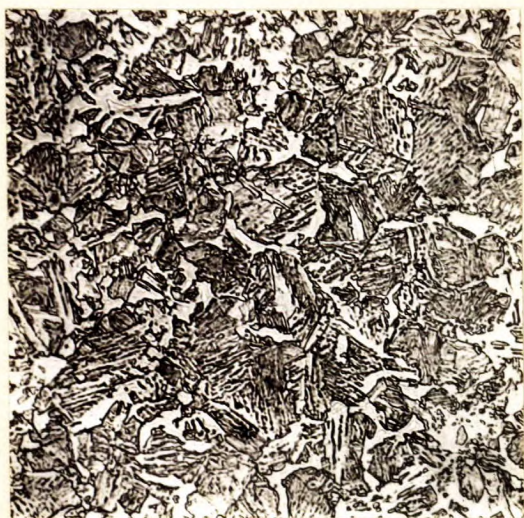
X500, nital etch. STRUCTURE OF PIN CORE. Low-carbon martensite and ferrite.
