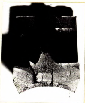
WESTINGHOUSE OPEN GATE PRODUCTION, SHOWING LESS FIBROUS STRUCTURE AND DEEP PENETRATION OF BRONZE.
