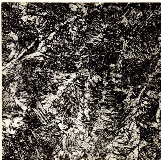
X100, nital etch. WELD METAL, HUB SECTION.
