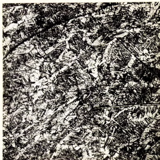
X100, nital etch. HEAT-AFFECTED ZONE, HUB METAL.
