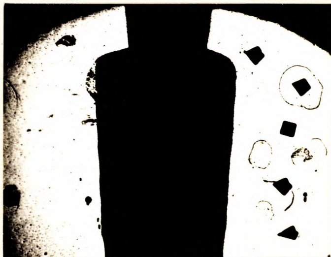
X30. CROSS-SECTION OF BEARING PIECE. Note absence of any evidence of wear.
