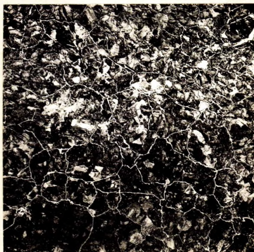
X100, nital etch. 0.41 PER CENT CARBON: GRAIN SIZE, 1-3.
