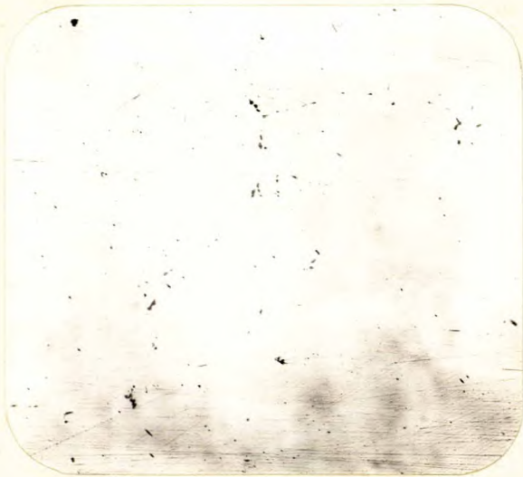
X100, unetched. PHOTOMICROGRAPH SHOWING EUTECTIC SULPHIDE INCLUSIONS.
