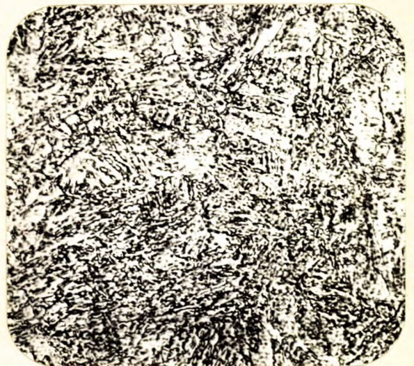
X1000, etched in 2 per cent nital. MICROSTRUCTURE: Tempered martensite. HEAT TREATMENT: Water-quenched, 1600° F.; Drawn, 1000° F.
